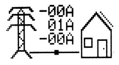
From top to bottom the display shows the measured values for L1, L2 and L3. A minus indicates that the power at that phase is delivered to the grid.
