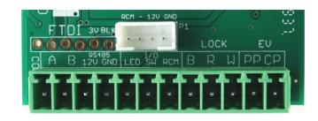
Connect the Sensorbox wires to terminals A, B, 12V and GND of the SmartEVSE.
